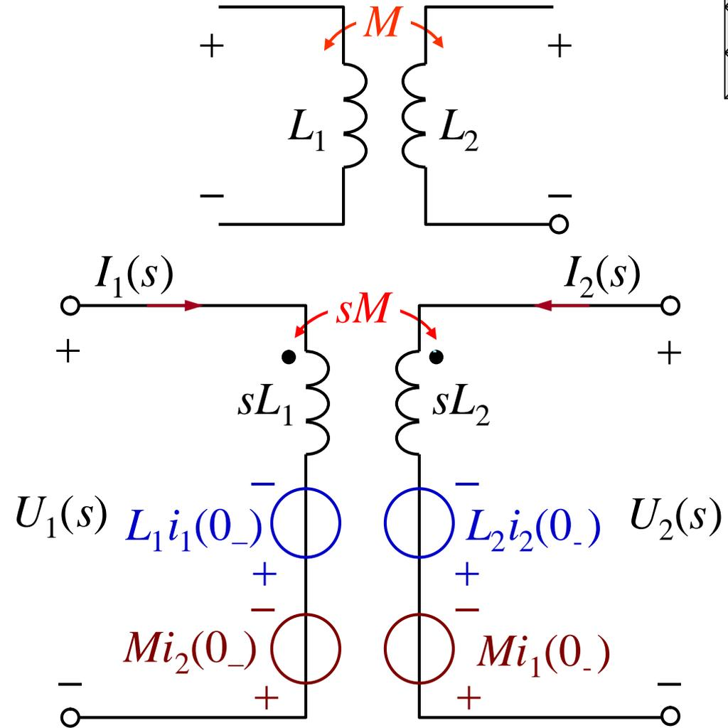
$$U_1(s) = sL_1 I_1(s) - L_1 i_1(0_-) + sM I_2(s) - M i_2(0_-)$$
